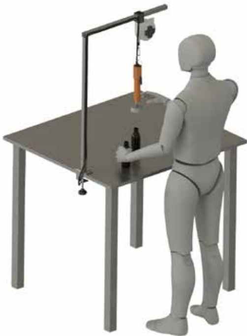
Semi-automatic capping with the aid of operator. The cap tightener is positioned immediately after the filling station, suspended in a hanger with a balance block for ergonomic handling. A cap tool adapted to the customer's caps is supplied with the cap tightener. A solution that works at a workbench or rotary table, or above a conveyor
