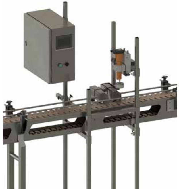
Automatic capping with manual lid placement. Automatic closure station comprising Queue & Positioning and cap tightener with cap tool mounted on a stand. The vertical movement of the cap tightener takes place automatically upon a signal from the sensor included. Placement of caps is performed manually by an operator before the station.
