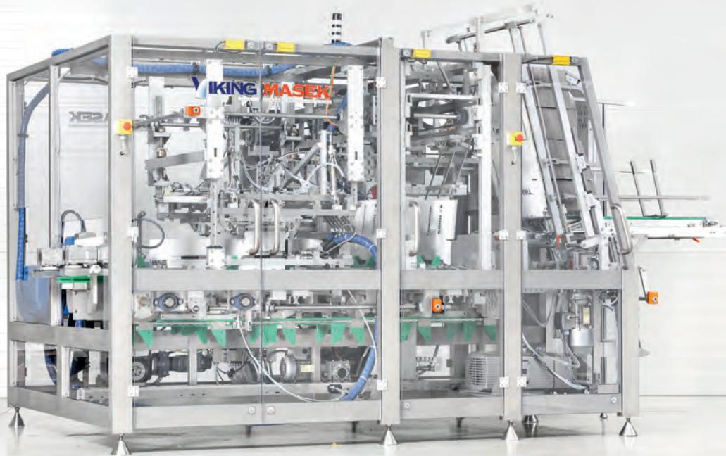
Viking Masek's CAM-W wrap-around cartoner is a fast paced machine that can collate and load products into wrap-around trays or cases. This intermittent motion cartoner features simple change-over for a broad range of applications and various customised feeders.
