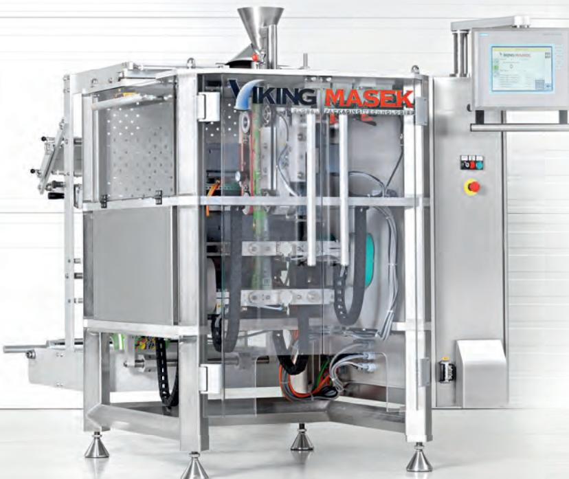
Patented, independently phased, twin sealing jaws separate the Velocity from all other high speed machines, and virtually eliminate lost cycle time. This is the fastest VFFS machine in the world – no competition.
