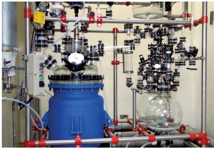
Distillation plant with 50 liters glass lined reactor and glass cover
