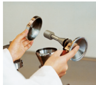
Open the vacuum tap and flame inside the funnel. Close the vacuum tap and flame the lid.
