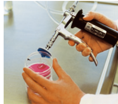
Wet the nutrient pads with 3.5 ml sterile and distilled or demineralized water
