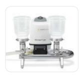
The Microsart® Combi.jet is a 2-branch manifold, made of high-grade stainless steel. The manifold has been specifically designed for the use together with the Microsart® e.jet Transfer Pump. The system is able to create sufficient vacuum for vacuum filtration concomitantly transferring the filtered liquid directly to waste. Microsart® Combi.jet and Microsart® e.jet can be easily connected and disassembled by the innovative Quick Connection technology.
