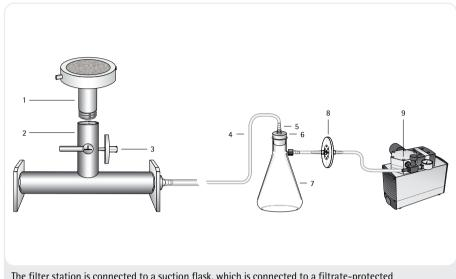
The filter station is connected to a suction flask, which is connected to a filtrate-protected vacuum pump.
