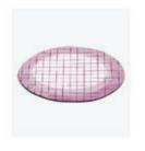
Hydrophobic edge membranes are used mainly for colony counting and sterility testing of solutions containing substances with antibiotic characteristics. The hydrophobic edge avoids the penetration of any growth-inhibitory substance into the membrane clamp zone wherefrom it could not be rinsed out and the substance could inhibit microbial growth during incubation.
