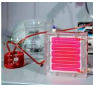
Vivaflow 200 set-up for diafiltration
