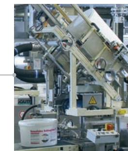
The closing machine takes up very little space as the lid magazine is arranged above the machine passage.
