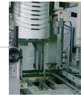
Full-surface separating segments separate the pails along the firm edge of the pail – a system which means the pails retain their original shape throughout the whole process.
