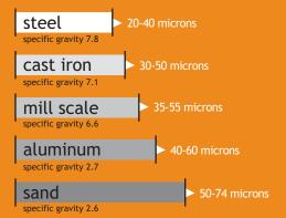
Flow rate & velocity are the key factors of LAKOS performance, creating centrifugal-action to remove particles heavy enough to be influenced by the g-force of this action. It is therefore logical that particle weight is the governing measure of LAKOS performance, translated to particle size by the chart above. Heavier particles are predictably easier to remove at smaller sizes.
