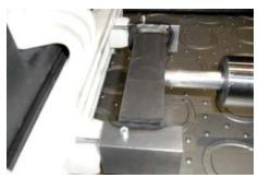
After the first half of the fixing clamp has been removed, the other side with the fixing pins can also be removed.
