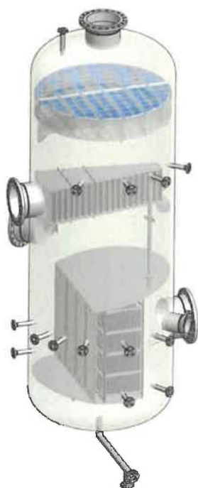
Isometric view of three-phase vertical coalescer/settler.
