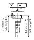
SensoGate® WA 131 Process adaptation for dairy pipe, DIN 11851, DN 50 ... DN 100, short and long immersion depth (ID)
