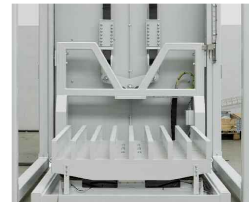
Movable compaction station with belt drive
