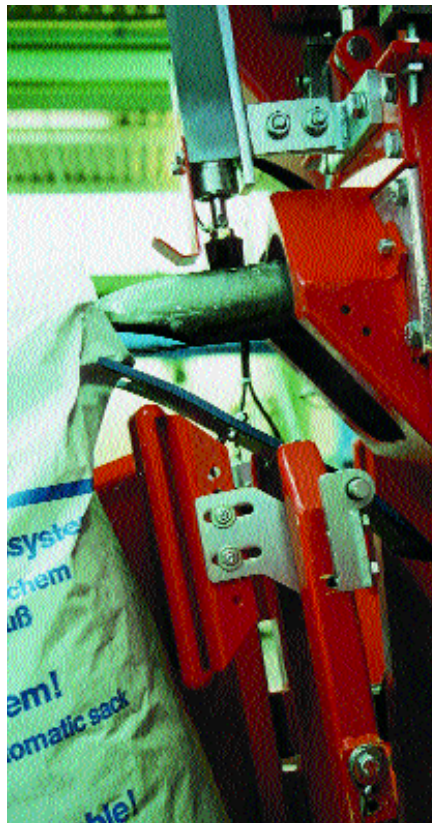
Spillage rejecting flap during bag discharge
