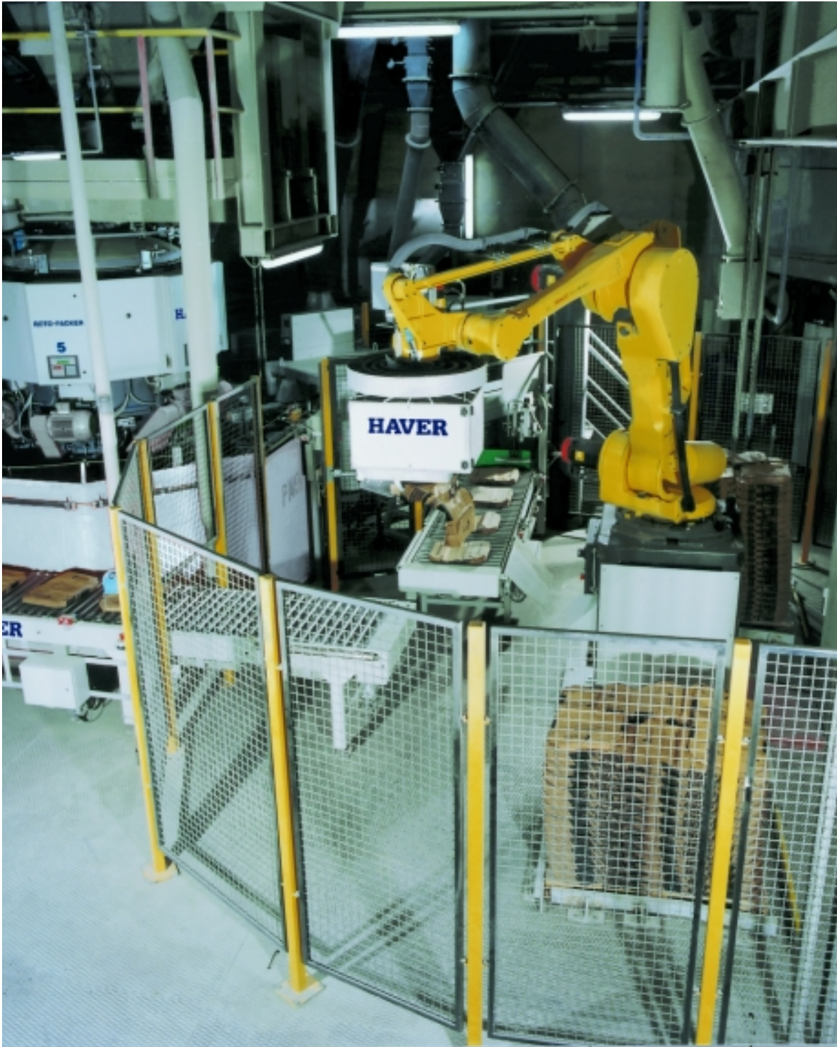
Depalletizing robot for empty bag bundles
