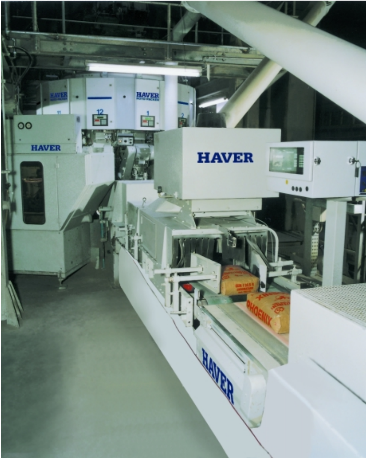
A Haver packing system with a Haver ROTO-PACKER, automatic bag applicator RADIMAT and check weigher
