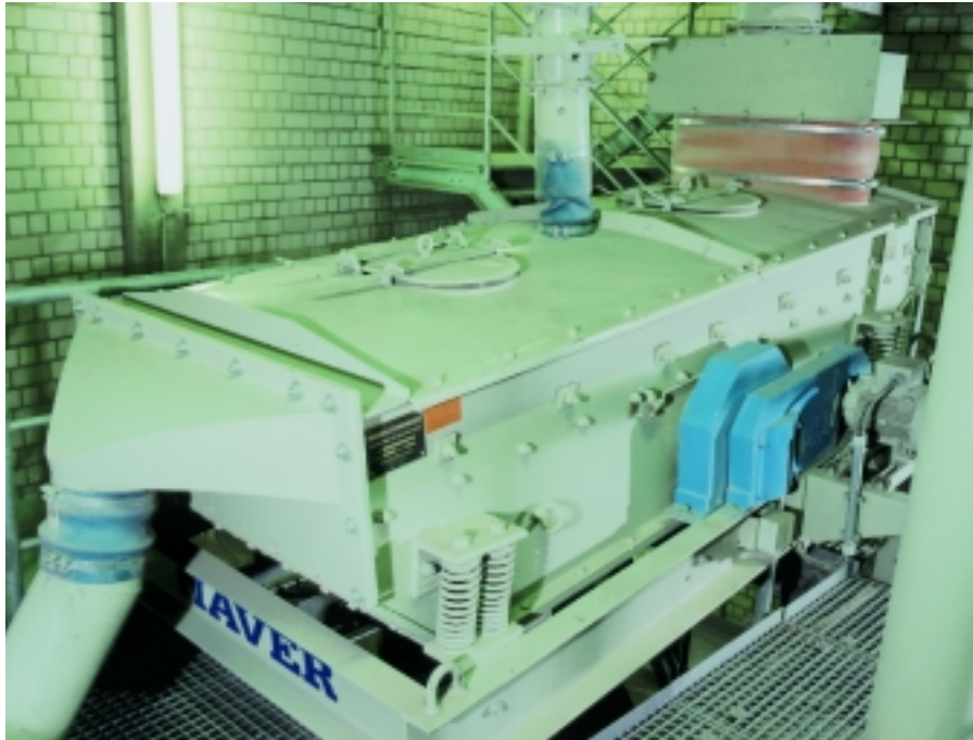
HAYER screens for foreign bodies in closed version (assembled)
