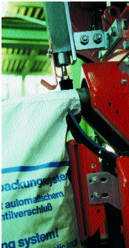
Spillage rejecting flap during filling process
