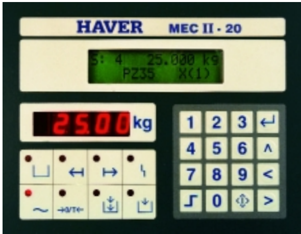
MEC II-20 operator terminal inside the ROTO-PACKER control cabinet
