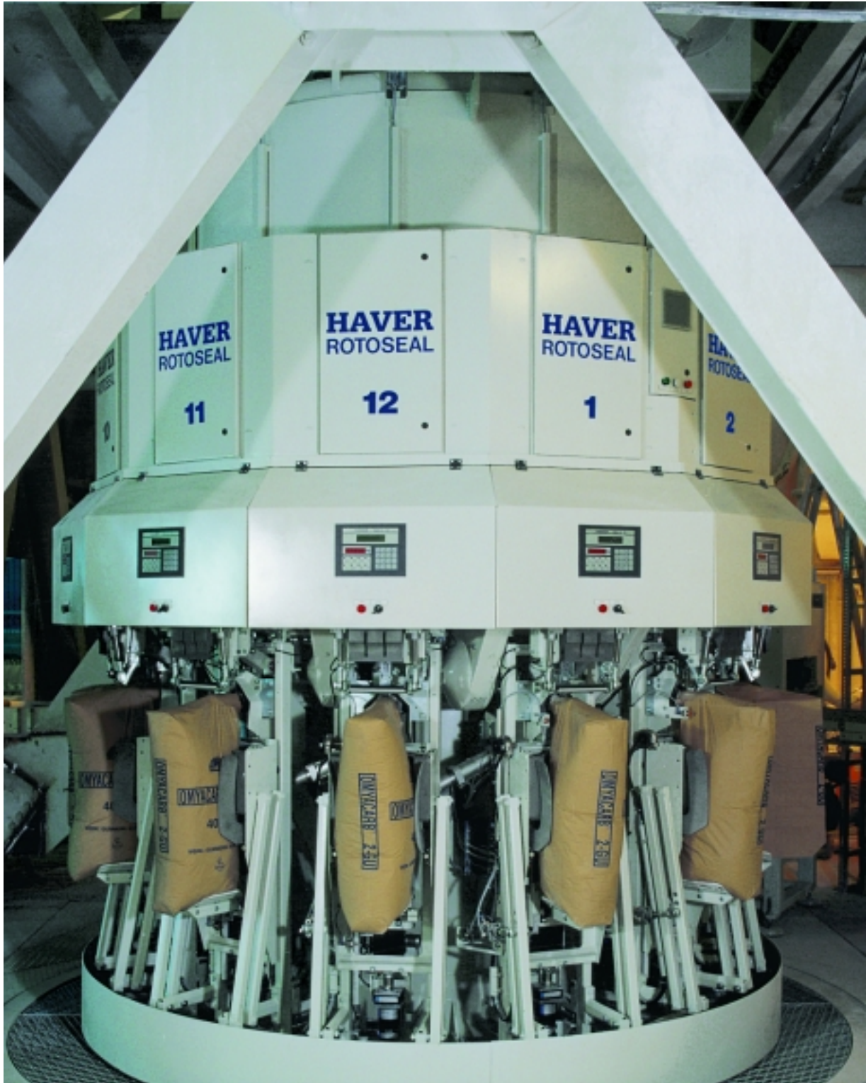
HAYER ROTOSEAL®-PACKER with valve sealing units
