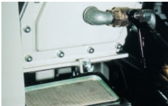
Cleaning trap door on filling vessel for an air type filling system (4)
