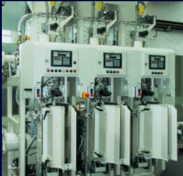
HAVER valve-type bag filling machine
