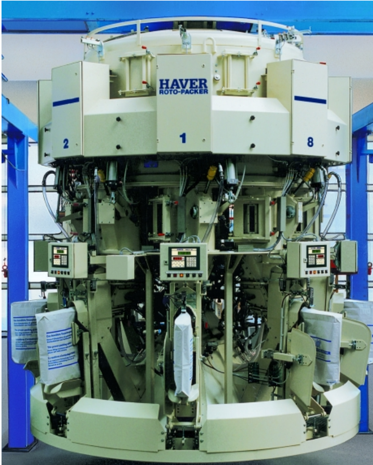
HAVER ROTO-PACKER type RLE with 8 filling spouts
