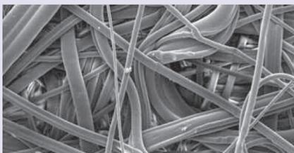
An innovative product manufactured with multiple layers of melt blown polypropylene media. This unique structure allows high flow rates while maintaining low differential pressure and ideal depth filtration characteristics.
