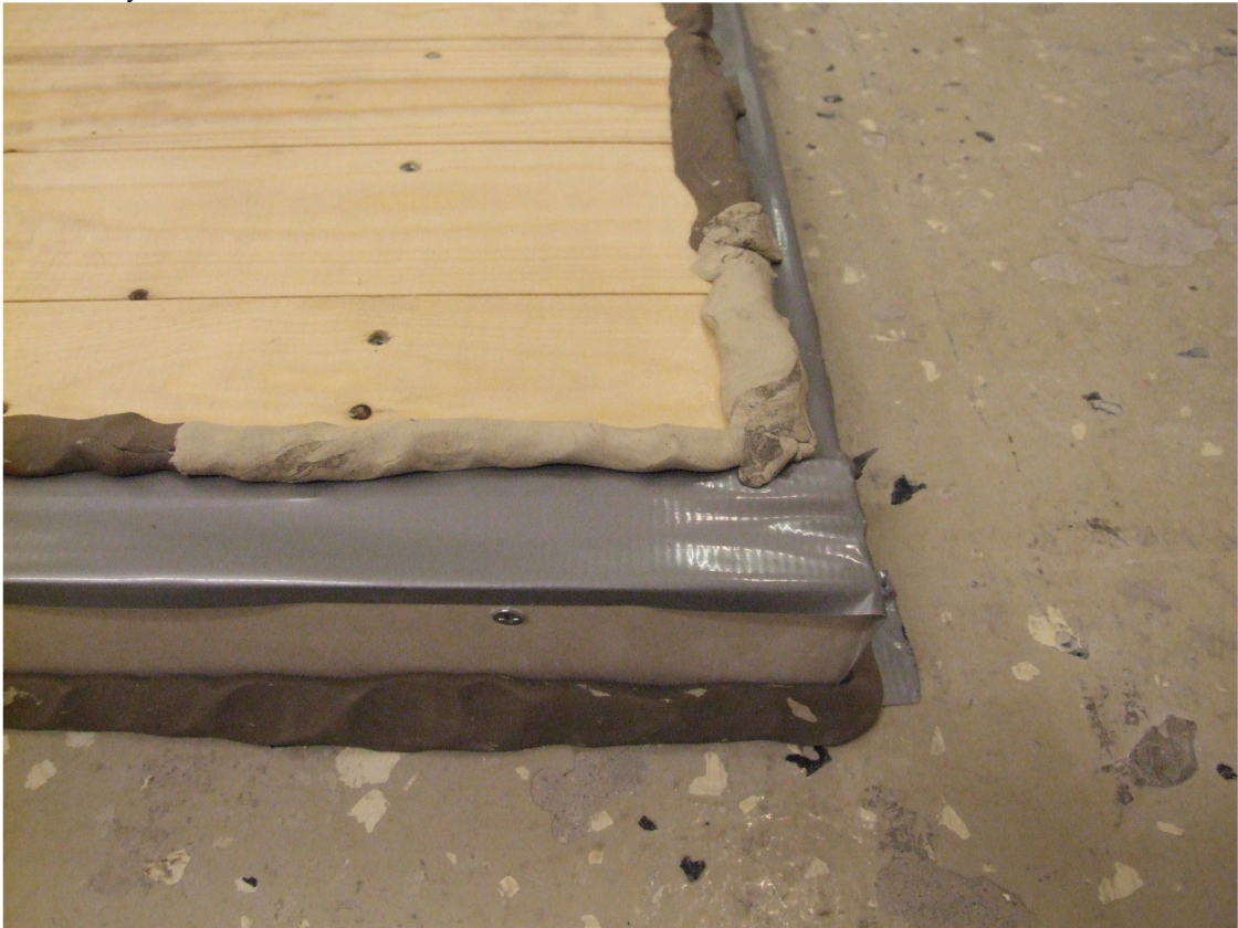
Figure 10 – Closing of the upper floor consisting of strips of gypsum board, tape and model clay.
