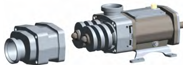
1. Removal of pump casing and cover
