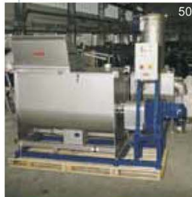
Clean charging of the double-screw mixer using EMDE sack discharger
