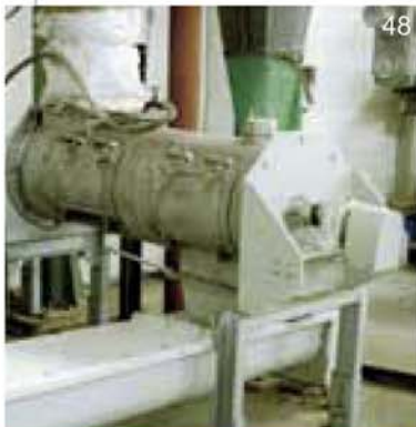
WUTRA paddle screw mixer for wetting sewage sludge
