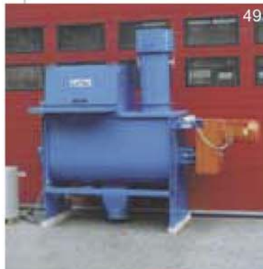
EMDE double-screw mixer with sack chute and filter
