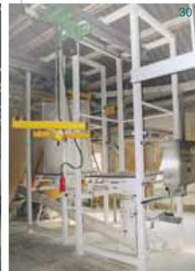
EMDE FIBC discharger with lifting device for the food industry
