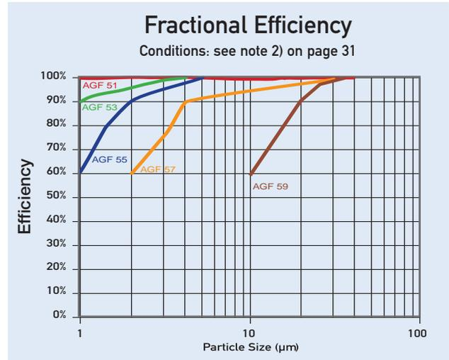
ACCUGAF Filter Bags, are available in retention codes of 51, 53, 55, 57, and 59. To select the perfect ACCUGAF Filter Bag for your application use the chart and choose the retention efficiency level you need on the left side of the chart at particle size in microns at the bottom. Next find which bag efficiency code (identified by the coloured lines) is closest to that point. There you have it, the most cost effective filter bag for your critical filtration application.
