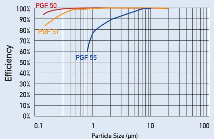
PROGAF Filter Bags are available in efficiency codes of 50, 51 and 55. To select the perfect PROGAF Filter Bag for your application, choose the micron retention efficiency level you need on the left side of the chart at particle size in microns at the bottom. Next, locate the bag efficiency code (identified by the coloured lines) that is closest to that point. There you have it: the most cost effective filter bag for your critical filtration application.
