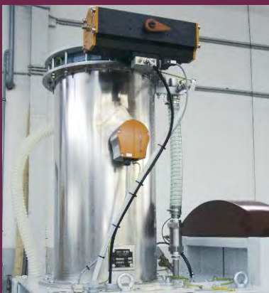
Filling chamber in electro-polished stainless steel design
