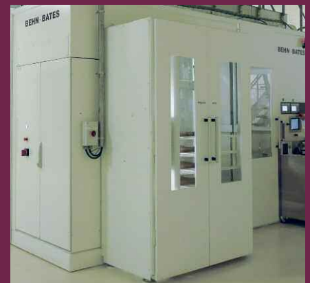
Vertical magazine integrated in the machine cabinet for better cleanliness and optimum space use
