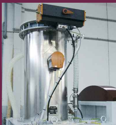
Filling chamber in electro-polished stainless steel design
