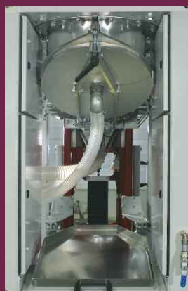
Chamber bottom: Closed and opened, with product spillage tray for easy and fast cleaning
