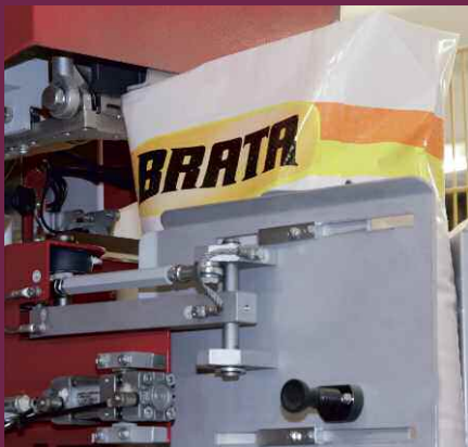
Valve bag sealing by ultrasound directly at the filling spout
