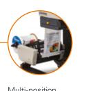
Multi-position unwind with tension control simplify changeover
