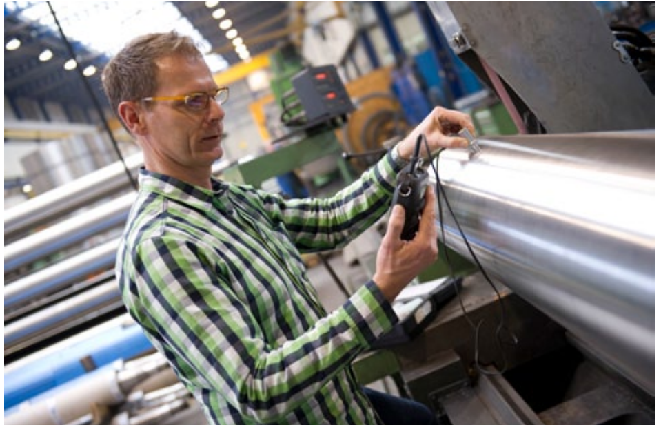
▲ Wall thickness measurement
