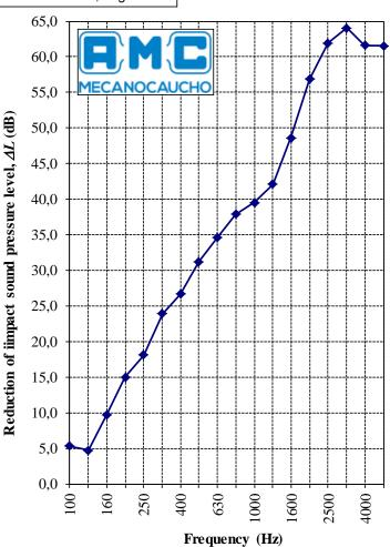
Weighted reduction of impact sound pressure level according to the standard ISO 717-2:2013
