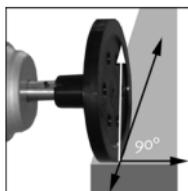
For speed and length measurement use the measuring wheel and keep the instrument in right (90°) angle to the moving direction of the material.
