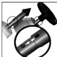
Place measuring cone tip, funnel tip or wheel onto the shaft – align pin and slot properly!
