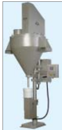
Bottom-up filler 400 litre capacity hopper to eliminate requirement for a surge hopper between the mixer and the filler Up-rated auger and agitation drive Pneumatic container lift system for bottom-up filling
