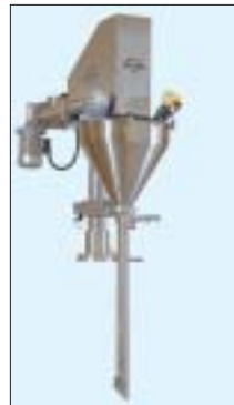
VFFS Vertical form-fill-seal configuration 56 litre seam-free hopper Long auger/funnel for dosing through forming tube Cut-off valve Horizontal auger hopper feeder for bulk feed from above Bracket-mounted with height adjustment
