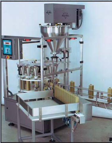
Indexing motion rotary system for vending drinks powders into canisters with extremely small neck opening, including checkweigher feedback and auto-stacking.
