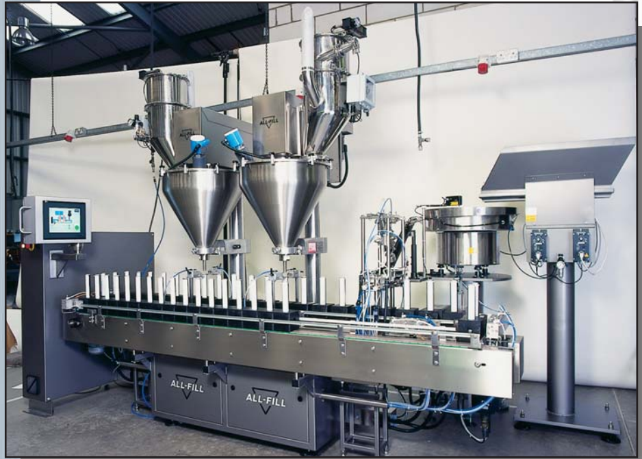
A puck indexing system for laser printer cartridges with tare and gross weighing, two stage filling, intermediate vibration, capping, weight/cap control, coding, single operator loading/unloading.
