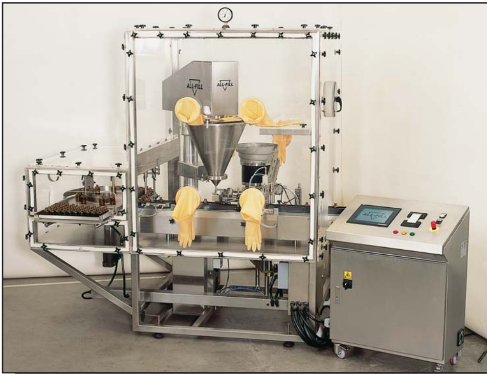
System for weigh-filling narrow-neck vials and bottles for the European Commission, with tray loading, rubber stoppering and integral isolation glove-box enclosure.
