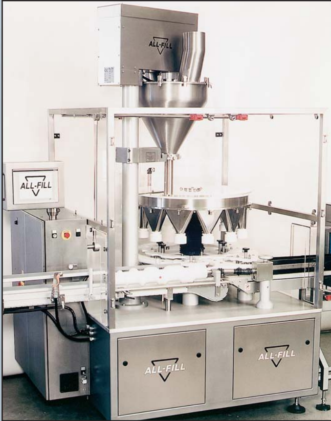
120 per minute spice filler with 500+ recipes held in memory for recall by product name/code
