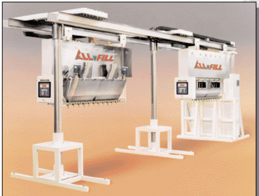
Duty/standby gantry installation with two 11 auger Multi-fills, 22 individually controlled servo drives with pre-selected acceleration/deceleration pattern, variable agitation speed to suit powder characteristics, complete with checkweigher feedback.
