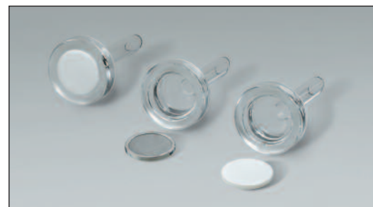
Glass frit, stainless steel support, PTFE support
