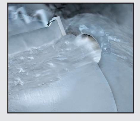
activated, energetically blowing on the bottom, fluidizing the residual product heel and making it available to be removed as part of the pneumatic transfer. It is possible to discharge 100% of the product left on the bottom of the vessel.
